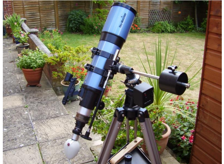
The author's Startravel 102mm fitted with a Vesta Webcam
