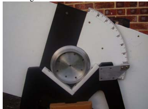
The Alt (up and down) Setting Circle
