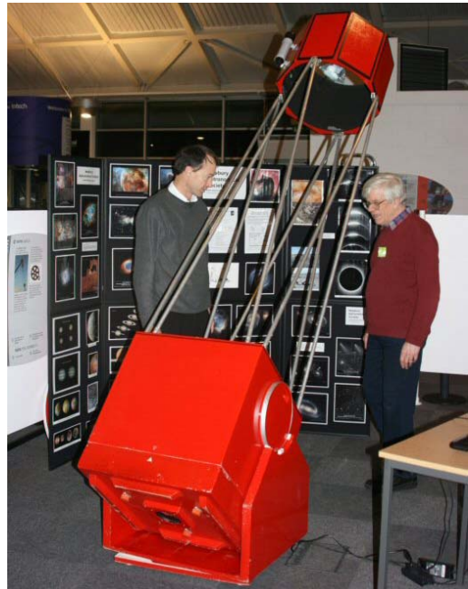
Richard Fleet's 20" Open Truss Tube Dobsonian
