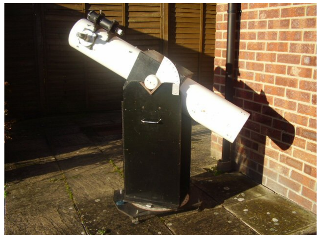
Steve Harris' 6" home made Dobsonian telescope
