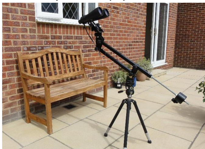
A Parallelogram Binocular Support with 15 x 70 fitted
